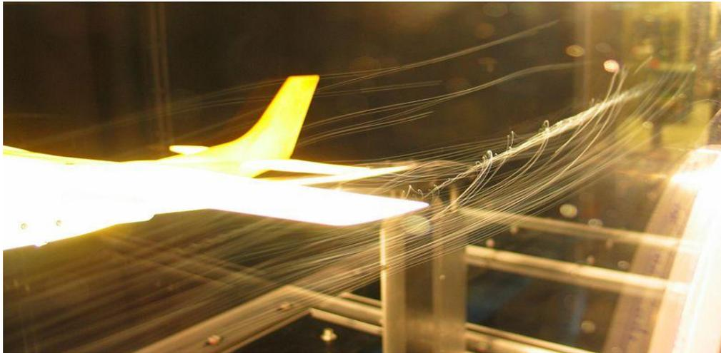
In the picture above, it can clearly be seen that the air is spiralling and trailing from the wing tip. This could create problems to the runway on take off by sucking up debris into the engine or affect the planes stability on landing.
