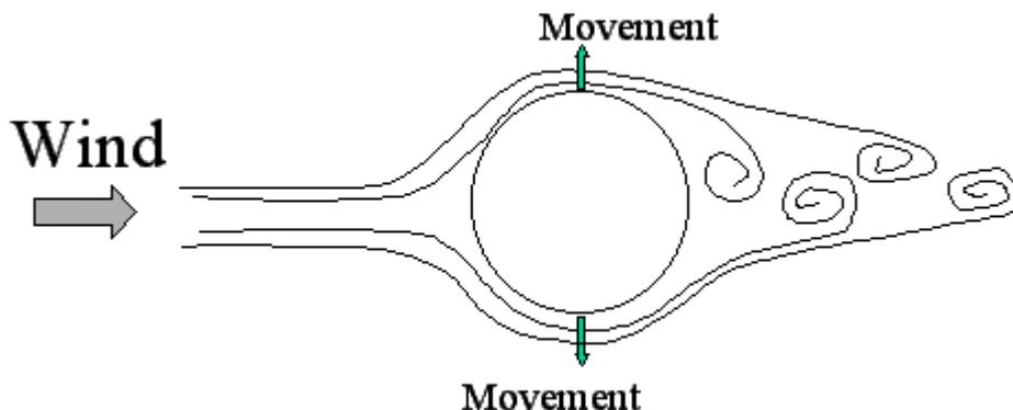
The diagram above shows that as the vortices are created, the structure experiences low pressure at certain places that excites movement. If this movement is, more than the structure can cope with then failure will occur.
