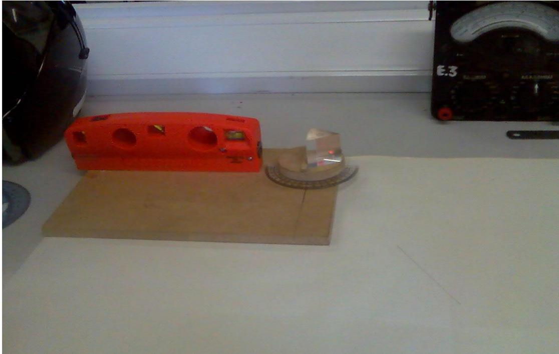
*[Fig 1.2 shows how light is refracted in a 60° prism]*
